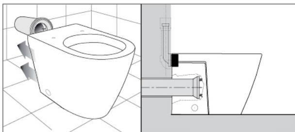
Push pan back into position. Ensure that you make a firm connection with inlet and outlet pipes and avoid disturbing the floor fixing brackets. Flush test for leaks.
