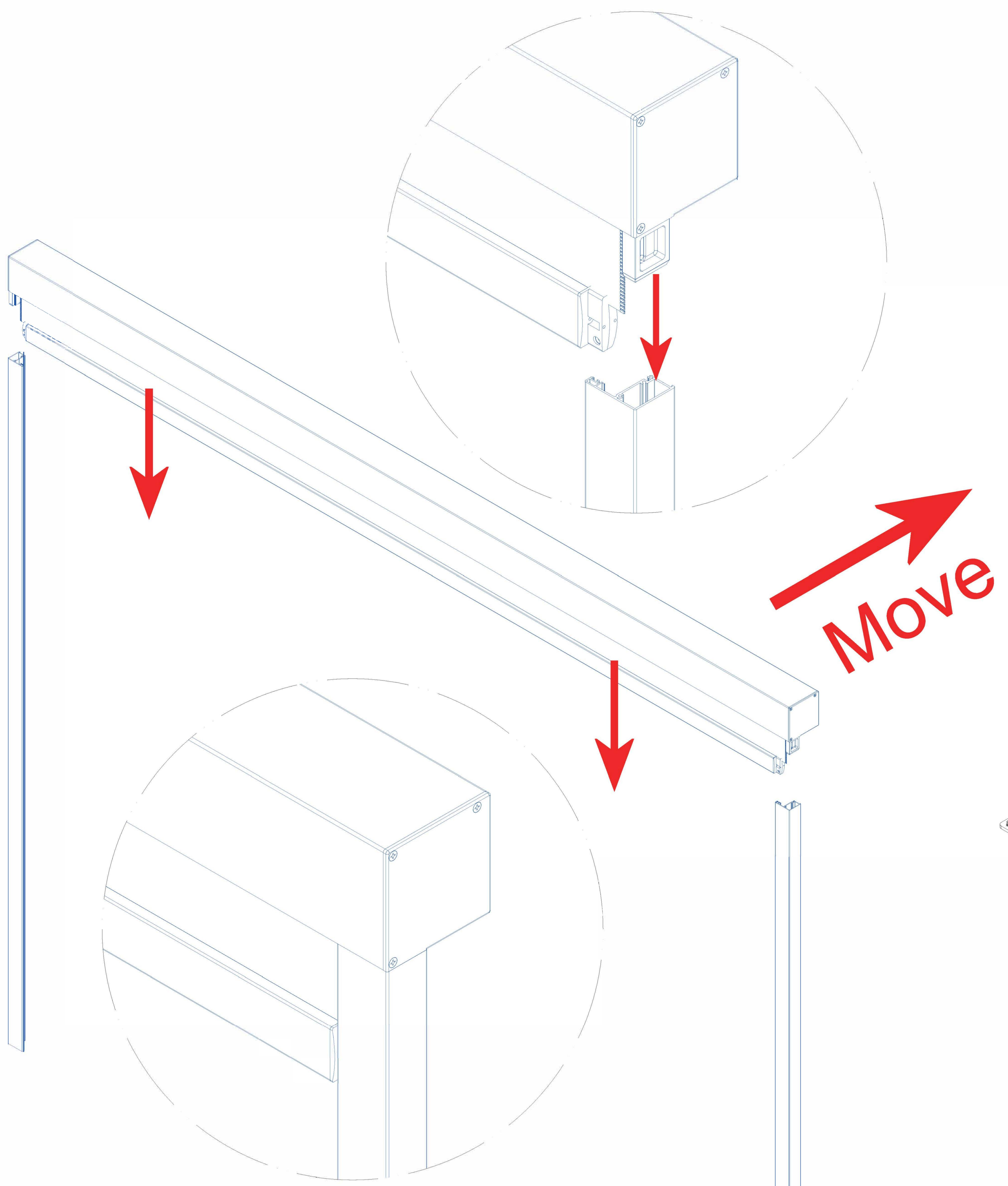
1. Please lift the support bar and the side curtain cover and insert the plastic part at both ends of the support bar in the rail.
